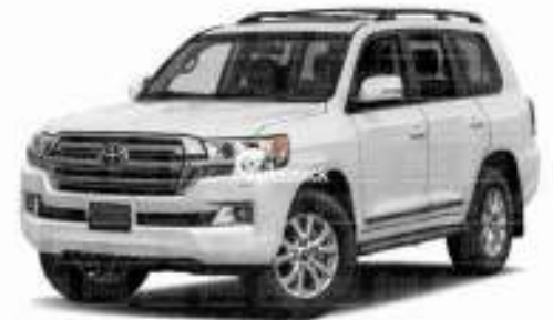
TOYOTA TWINTURBO LANDCRUISER V8 MOTOR: 1VD-FTV 4.5L
